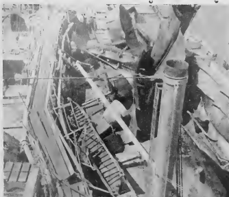
A torpedo ripped up the deck of the Esso Aruba when it exploded inside the ship.
